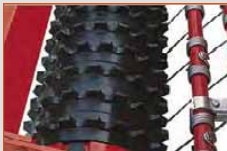
Corrugated roller with nylon/fiberglass rings to compact the ground for optimal seed germination
