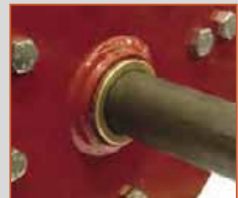
Both hub flanges are welded and equipped with two bronze bushings per rotor
