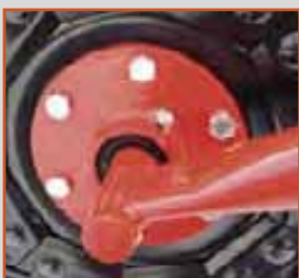
Cast steel hubs with greasable tapered bearings
