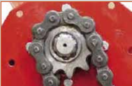
Lateral ASA 80 chain drive transmission in oil bath
