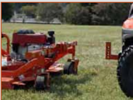
Front mount application with 2" receiver hitch
