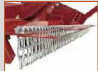
Chains provide safety from thrown objects
