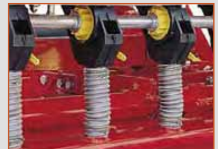
Precise seed metering cups
