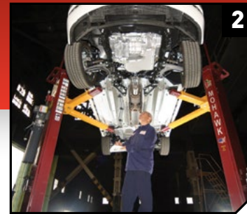
▲ Rotated columns with asymmetric lift arms will lift cars, trucks or vans with maximum safety and stability. 3" and 6" stacking adaptors included means no interference between lift arms and under vehicle access.
