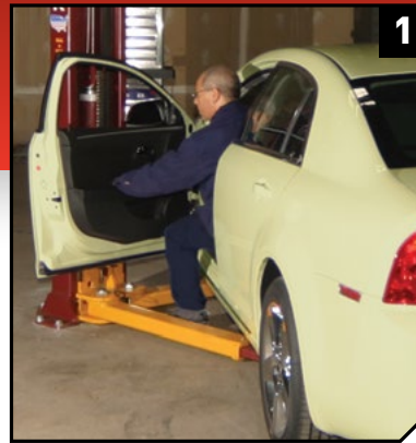
▲ Open any door on any vehicle for maximum clearance when switching from under-car to under-dash service.
