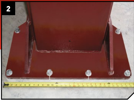
▲ Mohawk's large and stable footprint measures 30" wide by 24" and is made of 3/4" thick plate. Mohawk's large base gives stability to the lift, while distributing the load to the shop floor.
