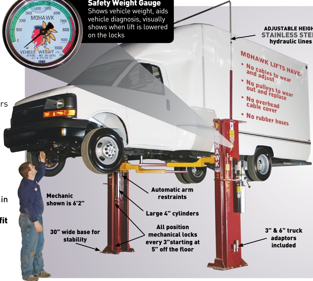
▲ Two post lifts offer FULL under vehicle repairs, takes up minimal bay space, while hanging free for tire, brake or any other need
