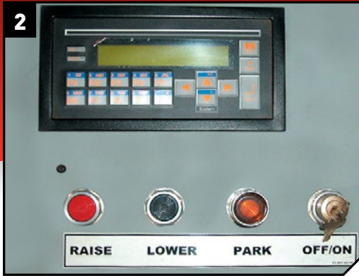
▲ Simple 3 button operation; Raise, Lower & Park (lock). 24 volt controls for operator safety, lockout standard, with easily programmed computer controls for fixed height jacks or used as a height limiter.
