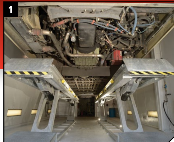
▲ Mohawk's clear work area has no obstructive tie bar between the runways for total access (galvanized lift shown).
