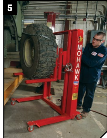
▲ Counterbalanced air-hydraulic tire dolly makes removing heavy truck tires a simple & safe one man job.
