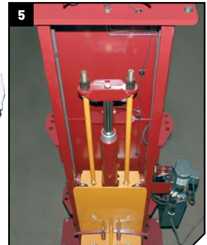
▲ Mohawk TP-20 columns are constructed of 1" thick, high strength fork lift mast channels, with 24 double sealed, self lubricating ball bearing rollers to smoothly raise the lift, using large 4½" cylinders for a lifetime of trouble free service.
