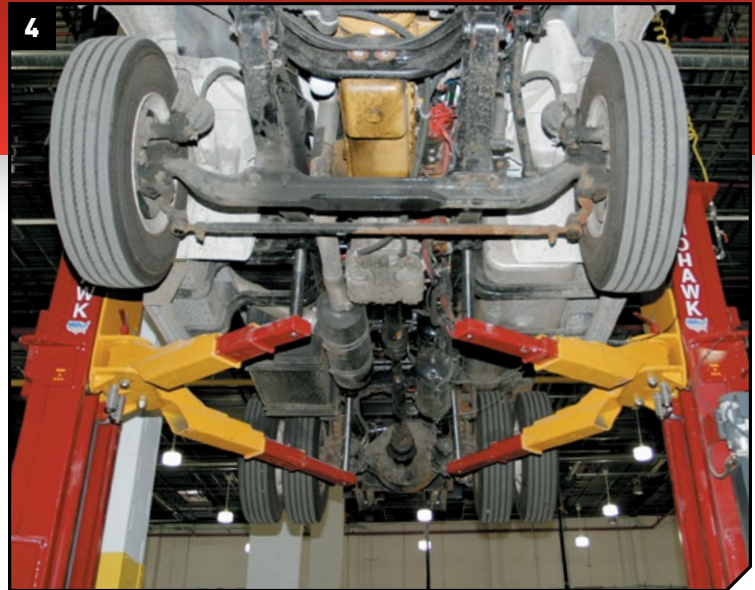
▲ Mohawk's TP-20 gives FULL under vehicle access for all repairs, takes up minimal bay space, while leaving the wheels hanging free for tire, brake or any other necessary repairs.
