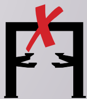
Mohawk lifts DO NOT use height restrictive overhead cable covers that limit lifting height.
