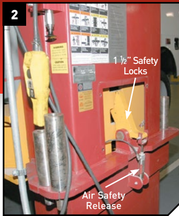
▲ Mohawk's all position mechanical and hydraulic safety systems lock the vehicles at ALL working heights. Mohawk safeties consist of 1 1/2" plate steel locks engaging into the slotted carriage lock racks every 6".
