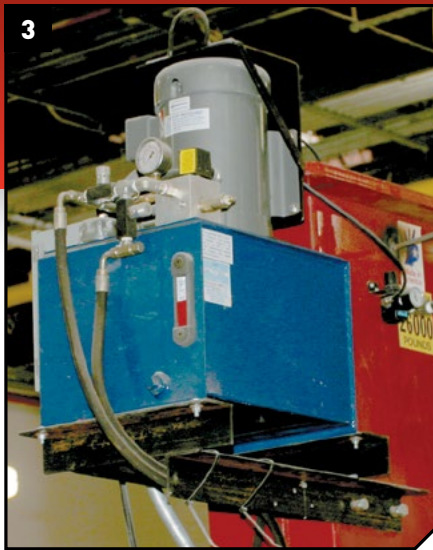
▲ 5 HP 3 phase power unit delivers fluid equally to twin hydraulic cylinders for quick and smooth lifting.
