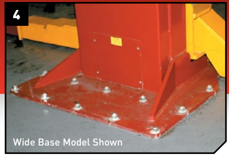
▲ Mohawk's large and stable footprint measures 48" wide x 30" (or 42") deep and is made of 1" thick plate. Mohawk's baseplate gives stability to the lift, while distributing the load to the shop floor. The TP-26/TP-30 requires 12" of concrete or optional footprint (shown) for shops with only 8" floors.
