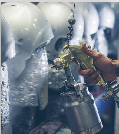
FOR PAINTED HELMETS, NEW PAINT IS APPLIED. PAINT COLOR CHANGES CAN ALSO BE MADE AT THIS TIME.
