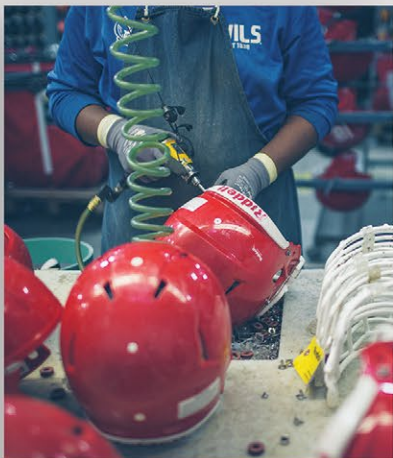
FACE MASKS, HARDWARE AND DECALS (IF APPLIED) ARE REMOVED.
