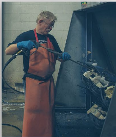
HELMETS ARE CLEANED AND SANITIZED BY HOT PRESSURIZED WATER AND DETERGENT AND THEN RINSED.
