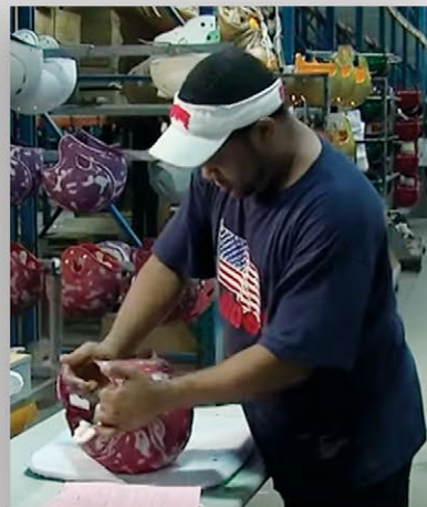
HELMETS ARE HAND-INSPECTED FOR HAIRLINE CRACKS AND ANY OTHER DEFECTS.
