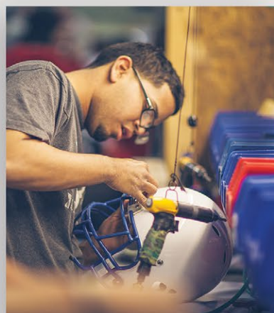
FACE MASKS AND HARDWARE ARE REATTACHED.
