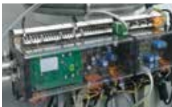
4 Central control unit AC
