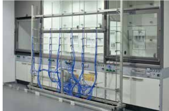
Fume hood control type approved under DIN EN 14175-T6 5.4 measurement in the exterior measuring plane
