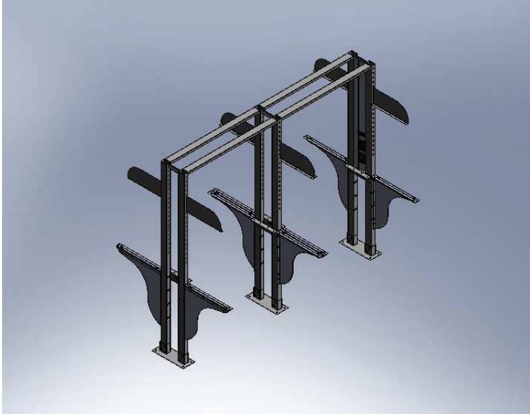
Discovery LT™ stand alone floor plate mounting system Floor plates, hardware, upper horizontal supports, and cantilevers where applicable are supplied.
