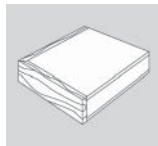
Laminate; 3/8" x 1-1/4" wood band edge; square corner; corner joint is not mitered (34S)
